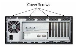
Remove all of these screws to open the enclosure.
